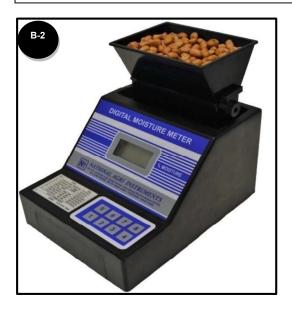
Now place the HOPPER on the top of the instrument/ meter so that KNOB & LEVER comes on the right side as shown. The alignment is important accuracy & repeatability.
