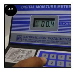
Press any switch 1, 2, 3, 4, etc. and check whether 'BAT' or 'LOBAT' appears on the left side of display. Insert the fresh pencil cells if 'BAT' or 'LOBAT' appears on the display.
