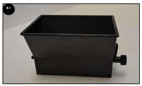
The HOPPER is provided along with instrument / meter and must be used to pour the sample in the measuring / seed compartment of the instrument.
