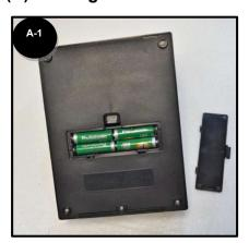
Locate the Battery compartment at the bottom. Insert the 4 X 1.5 V pencil cells if not there.
